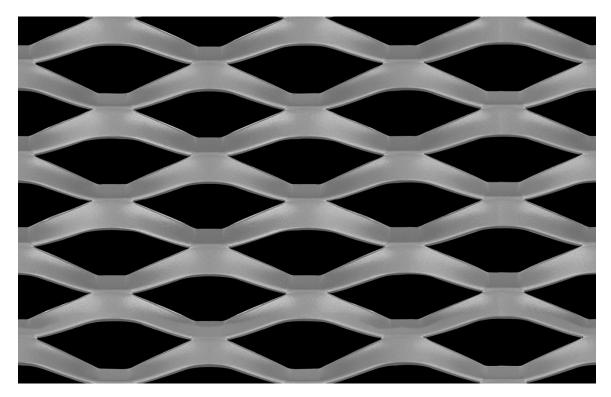
LW Pitch:50.80mmStrand Width:8.00mmSW Pitch:24.00mmThickness:1.20mmWeight:2.16 kg / m2Open Area:33%
